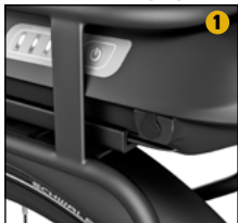
Location of charging
