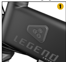
Location of charging
